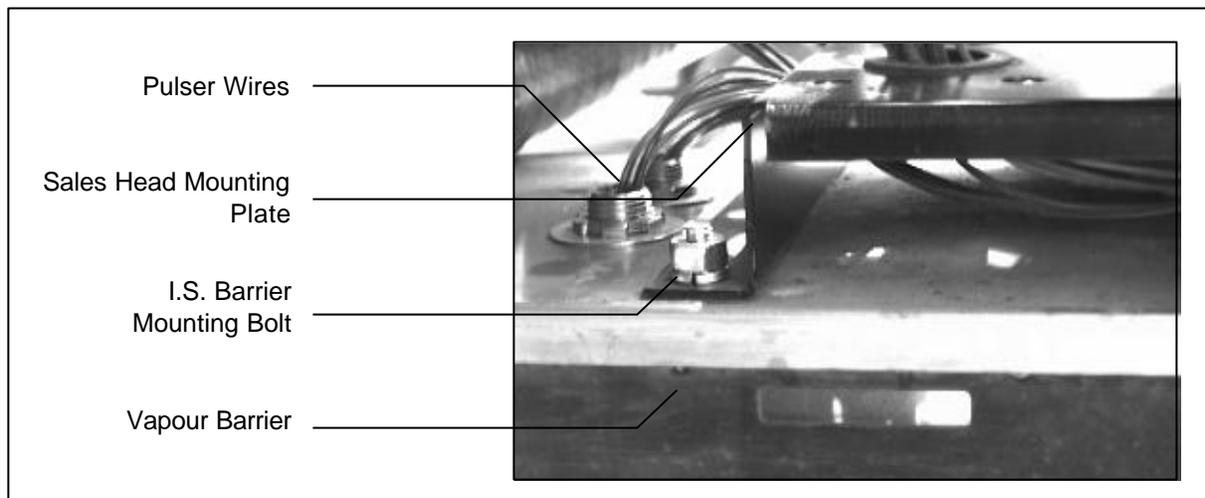
3. Connect corresponding probe plugs to I.S. Barrier via attached DIN jacks.
