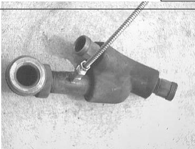
4. Install extension fitting (Part # BC 546) into hole, using sealing compound suitable for use with gasoline.
