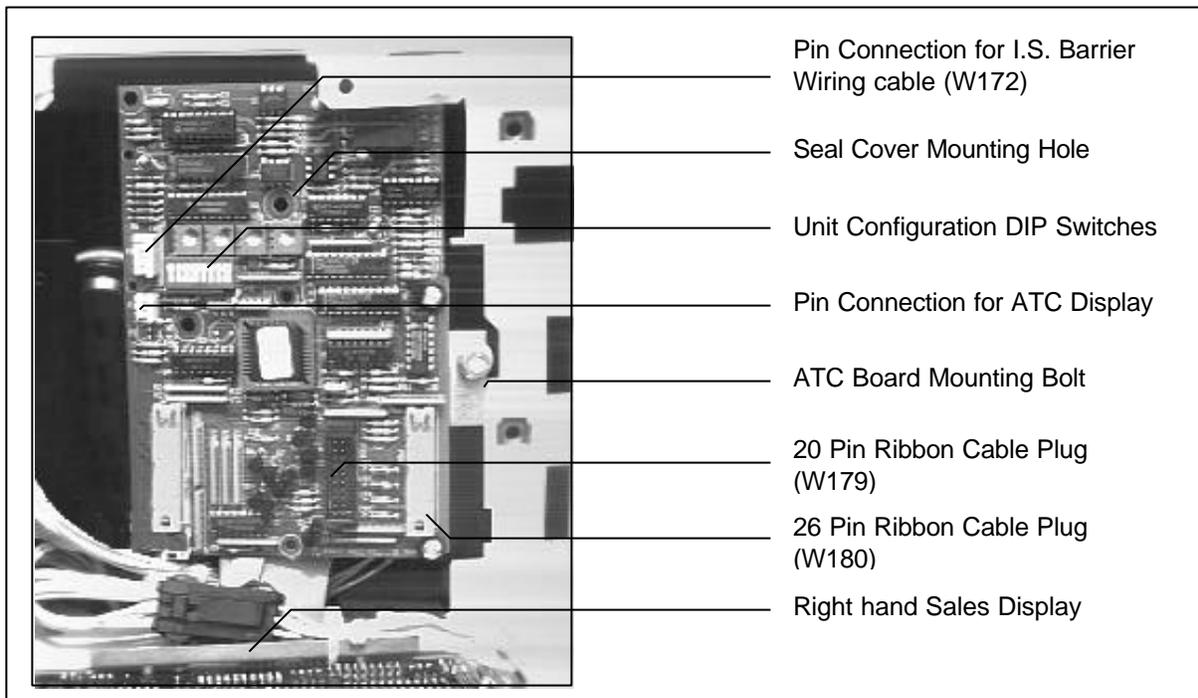
5. Connect the 20 pin ribbon cable (Part # W179) to the connector P106 on the ATC board, and run to connector P106 on the Modular Adapter Board, already attached to the Hydraulic Interface Board in the Card Cage.
